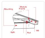
Clamp fitting: Using suitable module clamps on the LONG side of the module frame to mount the modules is "portrait orientation" mode, while on the SHORT side of the module frame is "landscape orientation" mode.
